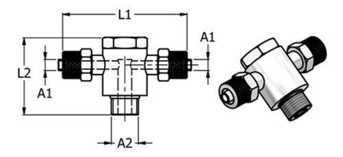
Hose diameter A1 = 5/3L1 = 33.0L2 = 17.5NV = 8Thread A2 = M5
